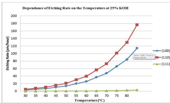
Fig. 3. Dependence of etching rate with temperature at 25 wt% KOH concentration
