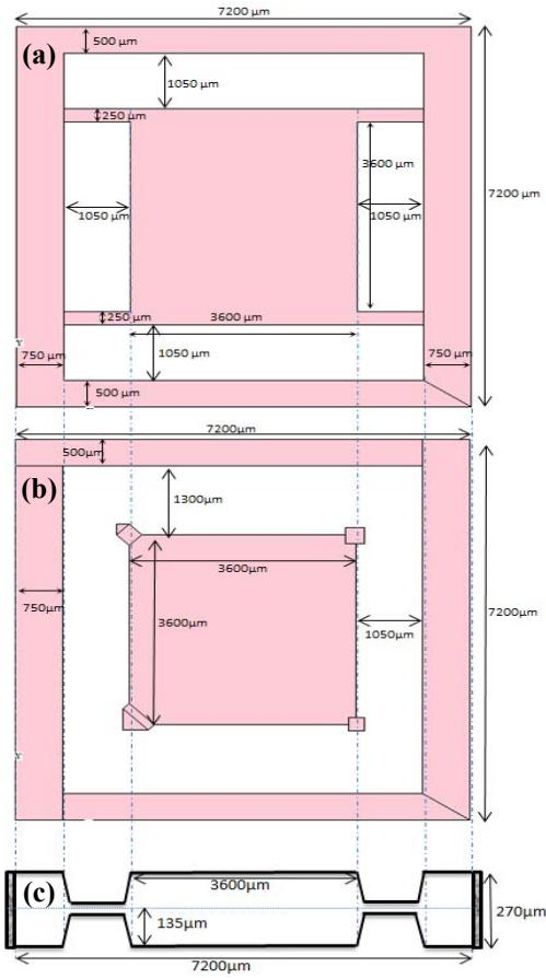
Fig. 1. (a) Top mask (b) Bottom mask (c) cross section view of complete accelerometer structure
