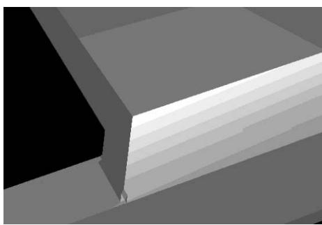
Fig. 7. Etched accelerometer structure with square corner compensation mask
