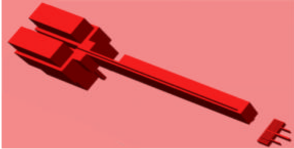
Figure 6 Solid model of a thermally actuated beam developed at Texas Christian University [8]
