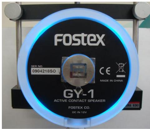
Fig. 6. Photograph of the experimental setup for vibrating the asymmetric silicon micro-mirror
