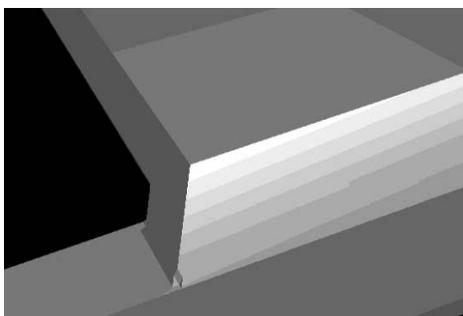
Fig. 7. Etched accelerometer structure with square corner compensation mask
