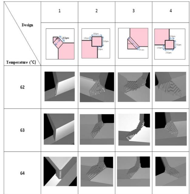
Fig. 4 Etched morphology of convex structure at 4.5 hours etching time at different etching temperature.
