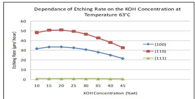
Fig. 5. Dependence of etching rate on KOH concentration at temperature 63 °C.
