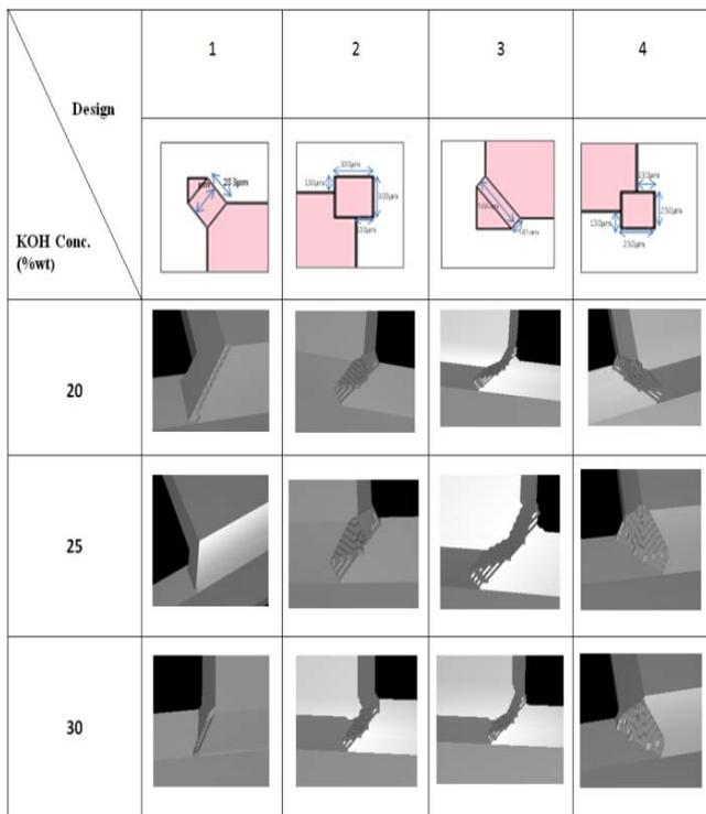
Fig. 6. Etched morphology of convex corner structure at 4.5 hours etching time at difference KOH concentration.
