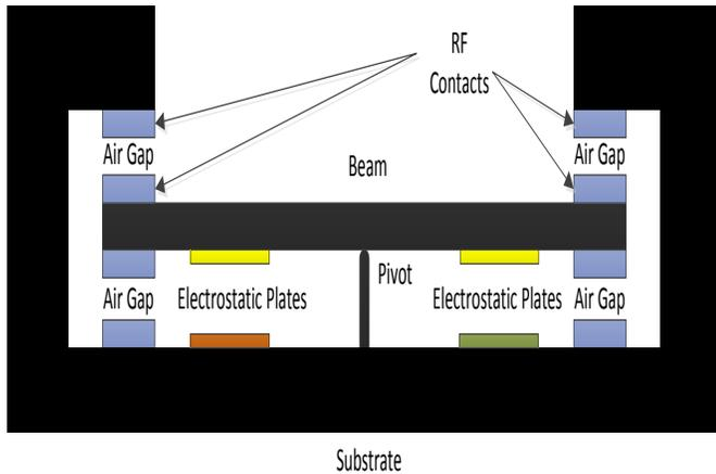
Figure 1: Cross sectional representation of the RF MEMS seesaw switch in the 'off-state'
