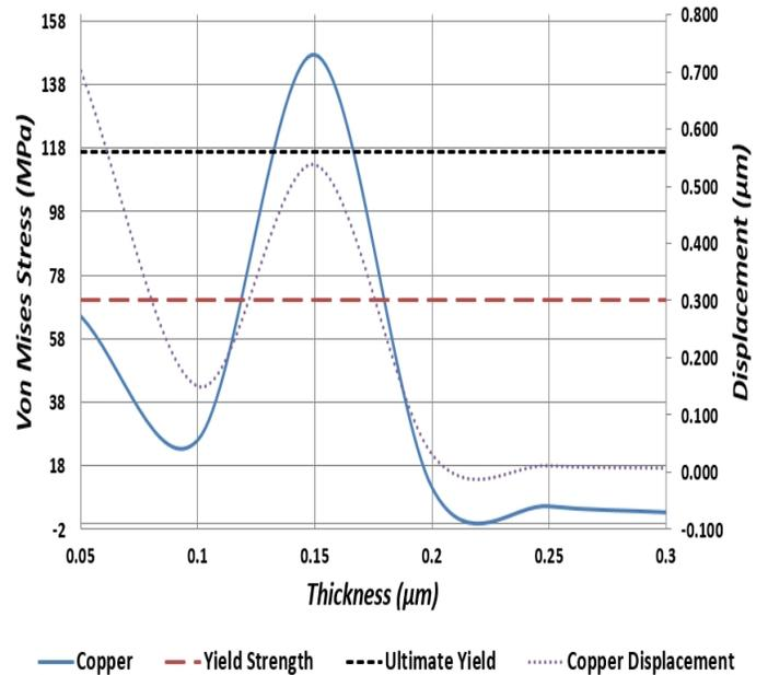
Figure 9: Von Mises Stress and Displacement vs Thickness of Copper pivot at 3V
