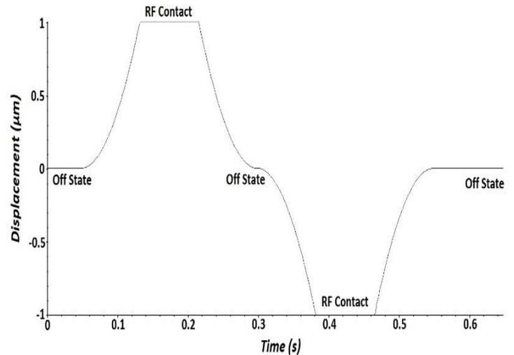
Figure 5: Displacement vs. Time using a copper pivot width of 0.048  $\mu\text{m}$
