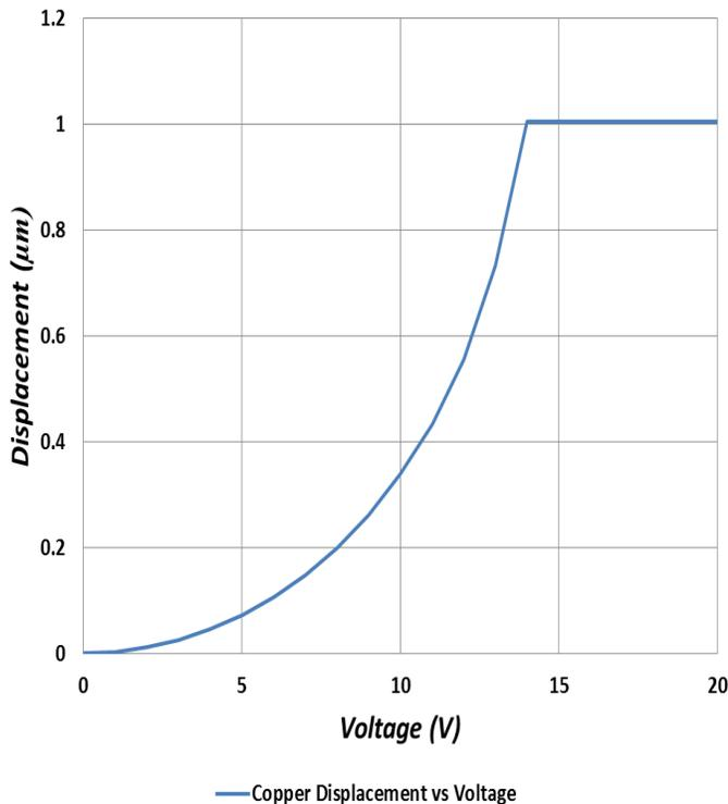
Figure 4: Displacement vs. Voltage for copper width of 0.048 $\mu\text{m}$
