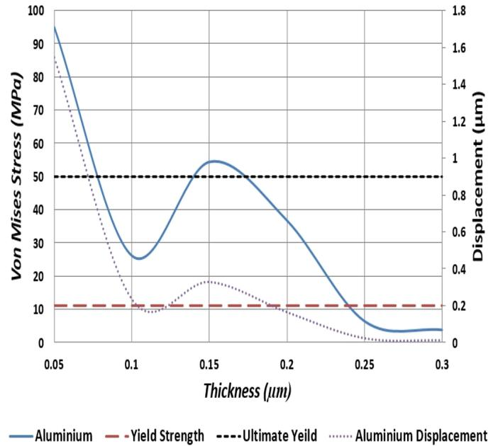
Figure 8: Von Mises Stress and Displacement vs Thickness of Aluminium pivot at 3V
