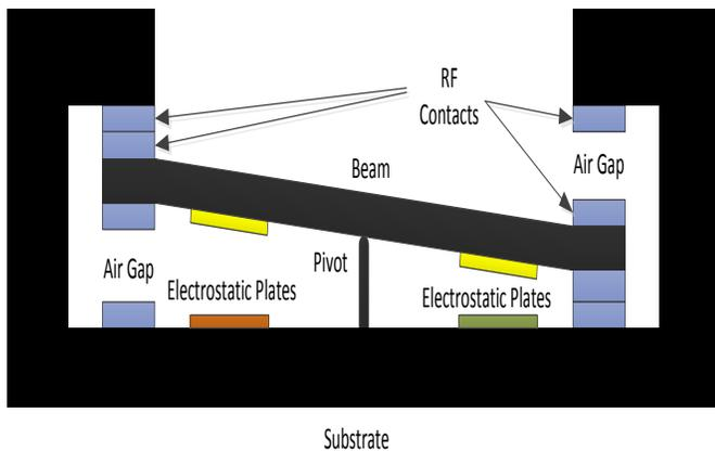
Figure 2: Cross sectional representation of the activated RF MEMS seesaw switch in the 'on-state'
