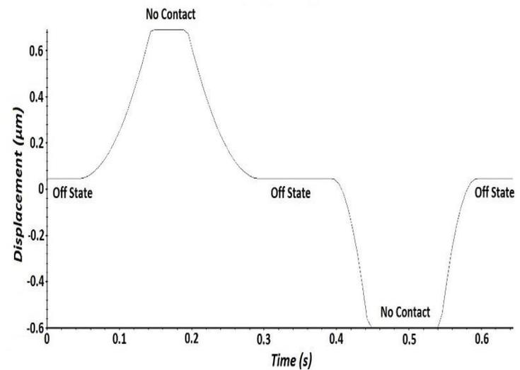
Figure 6: Displacement vs. Time using a copper pivot width of 0.053  $\mu\text{m}$
