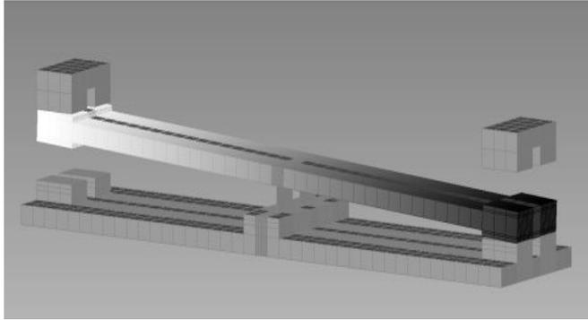
Figure 3: Activated RF MEMS seesaw switch. An early prototype simulation, of an oblique view in the ‘on-state’
