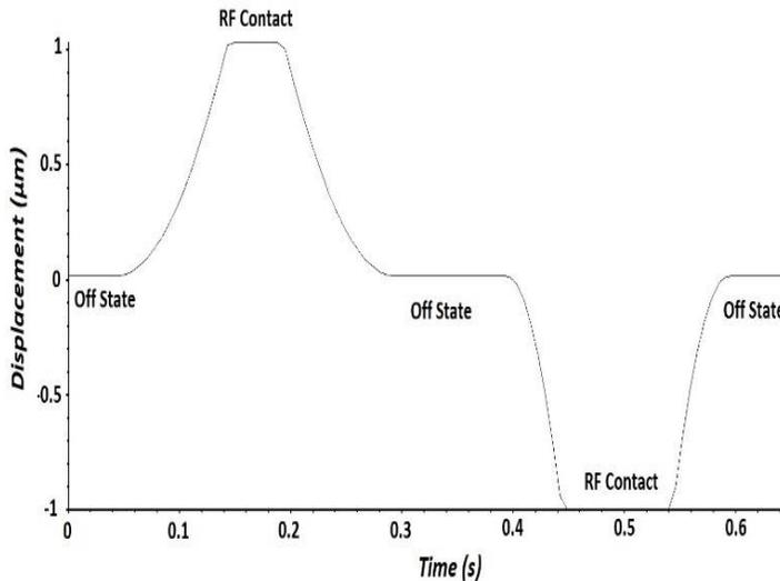
Figure 7: Displacement vs. Time using an Aluminium pivot width of  $0.053 \mu\text{m}$
