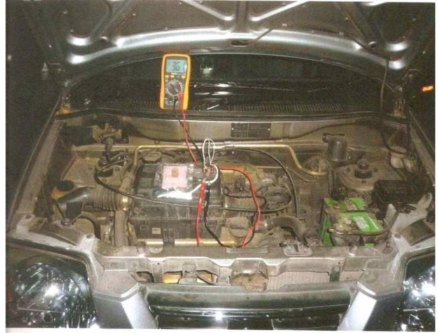
Figure12. PZT EHD mounted on the surface of the car engine
