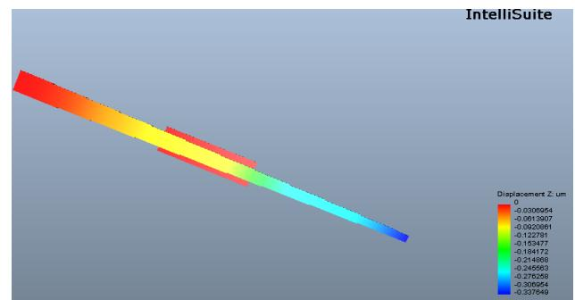
**Figure 8. Tapered V-Shaped Beam**
