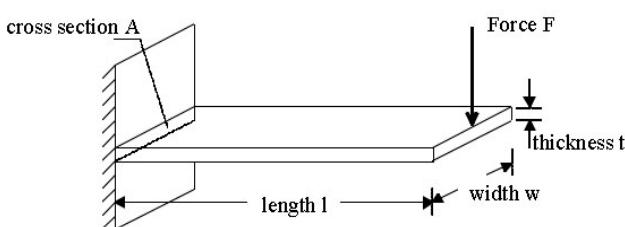
**Figure 5. Cantilever Structure with Labling**
