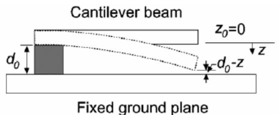
Figure1. Geometric model of cantilever
