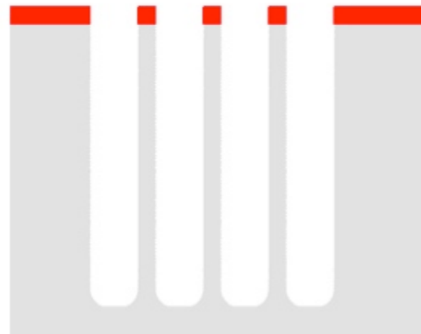
The experimental results of the etching. Comparison of etching 5 μm openings with an etch/dep cycle of 7s/7s.
