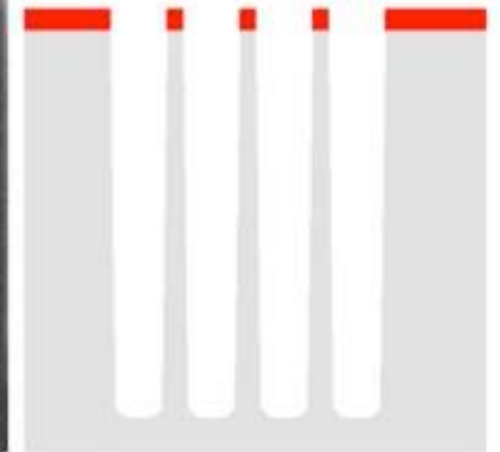
Comparison of etching a 5 μm trench with a 5s/7s cycle
