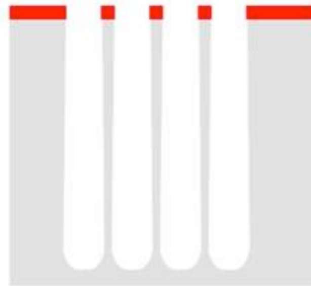
Comparison of etching a 5 μm trench with a 7s/8s cycle
