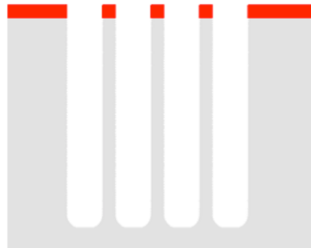
The experimental results of the etching. Comparison of etching 5 μm openings with an etch/dep cycle of 7s/7s.
