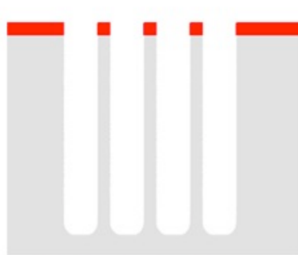
The experimental results of the etching. Comparison of etching 5 μm openings with an etch/dep cycle of 7s/7s.
