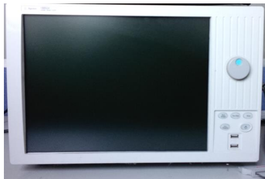
Semiconductor logical analyzer
